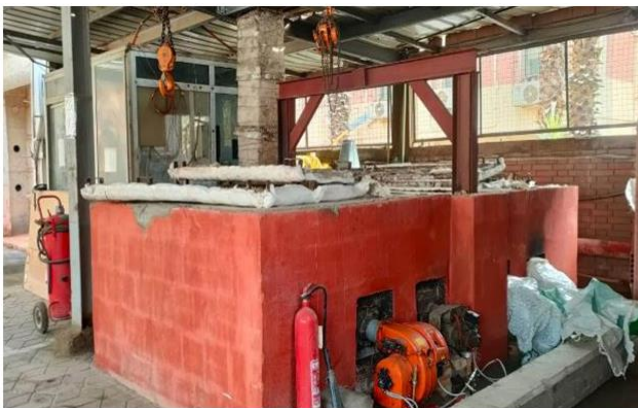
FIGURE 8. Testing furnace in HBRC fire lab
